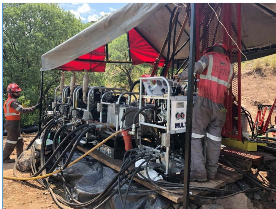
Figure 10.1 Man-Portable drilling rig at site of SJ21-01
