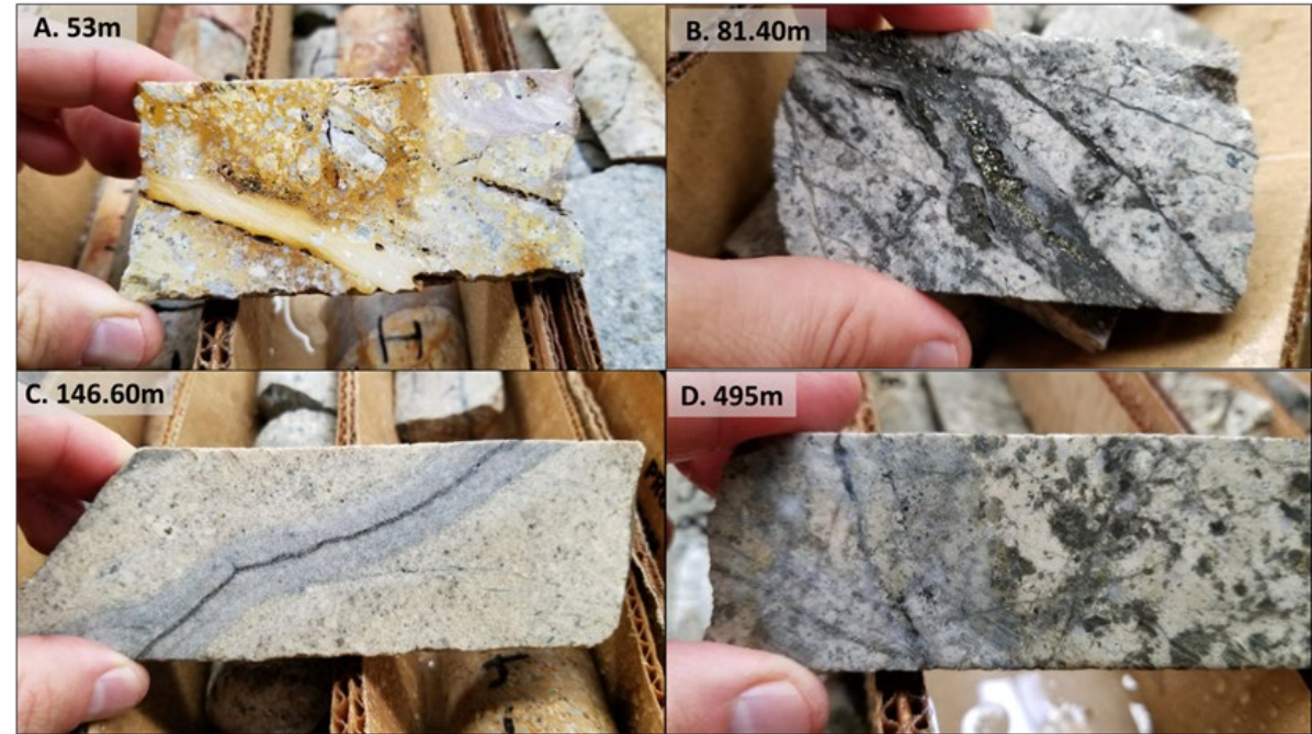
Core photos from historic IV-1 drill hole. A: FeOx zone with advanced argillic alteration; B: Transition AA -> PHY alteration with trace chalcocite and 6-7% pyrite; C: QSP vein; D: A and B veins with chalcopyrite, bornite and molybdenite.
