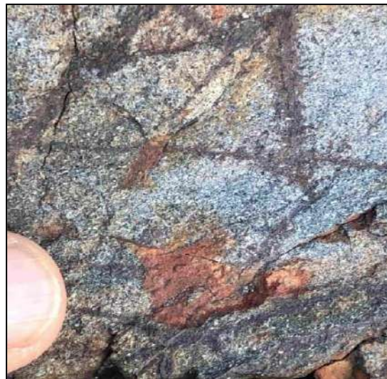
Figure 7-5: Fine-grained Andesite Dike; Field of View is Approximately 3.5 x 3.5 cm
