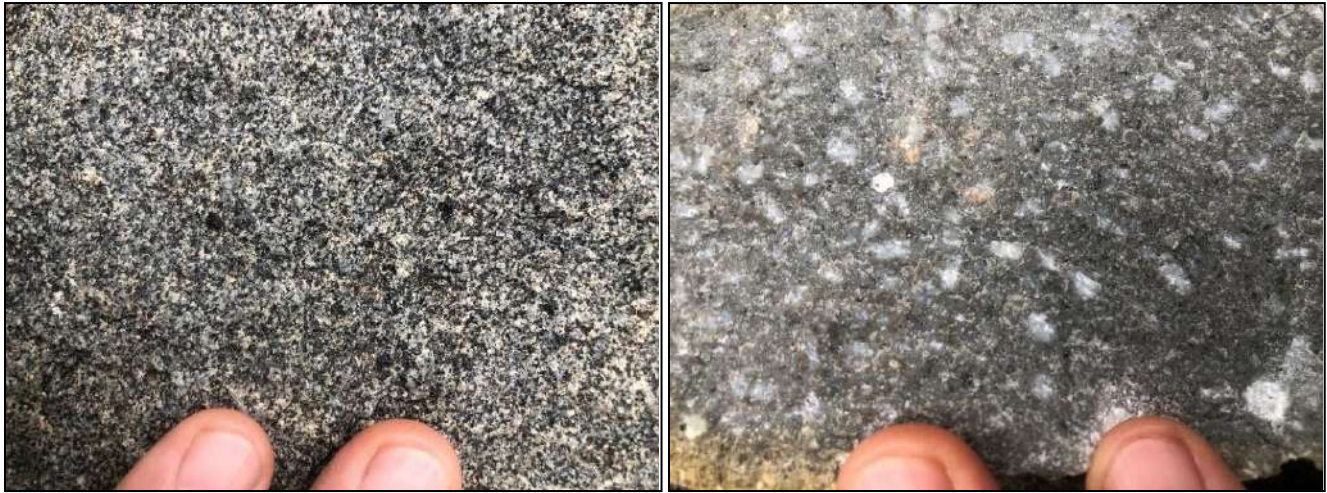
Figure 7-4: Pictures of a Fine-grained Diorite and a Monzonite Porphyry
